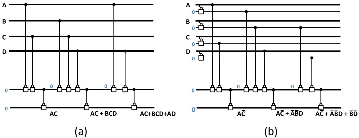
Figure 19. (a) Realization of Unate SOP with 2WMS, (b) Realization of general SOP with 6WMS
