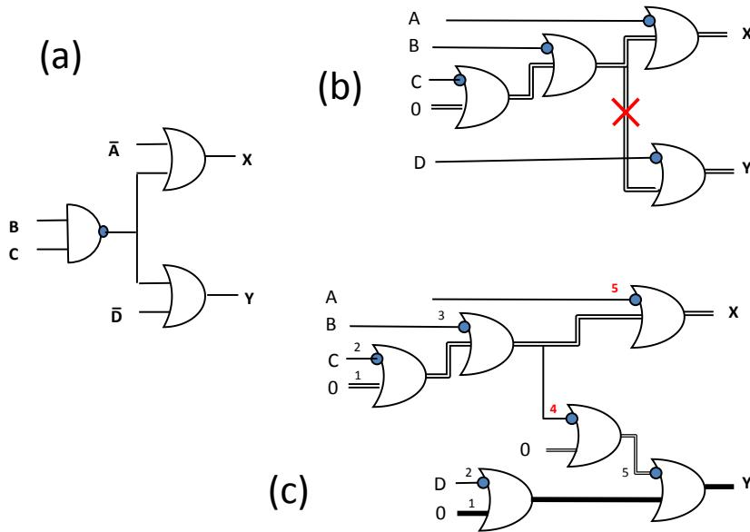
Figure 5. Fan-Out problem (a) NAND gate output going to two gates.
