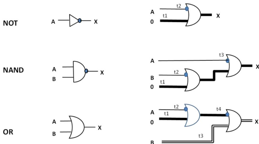
Figure 4. NOT, OR and NAND gates realized from IMPLY gates assuming that the inputs already exist.
