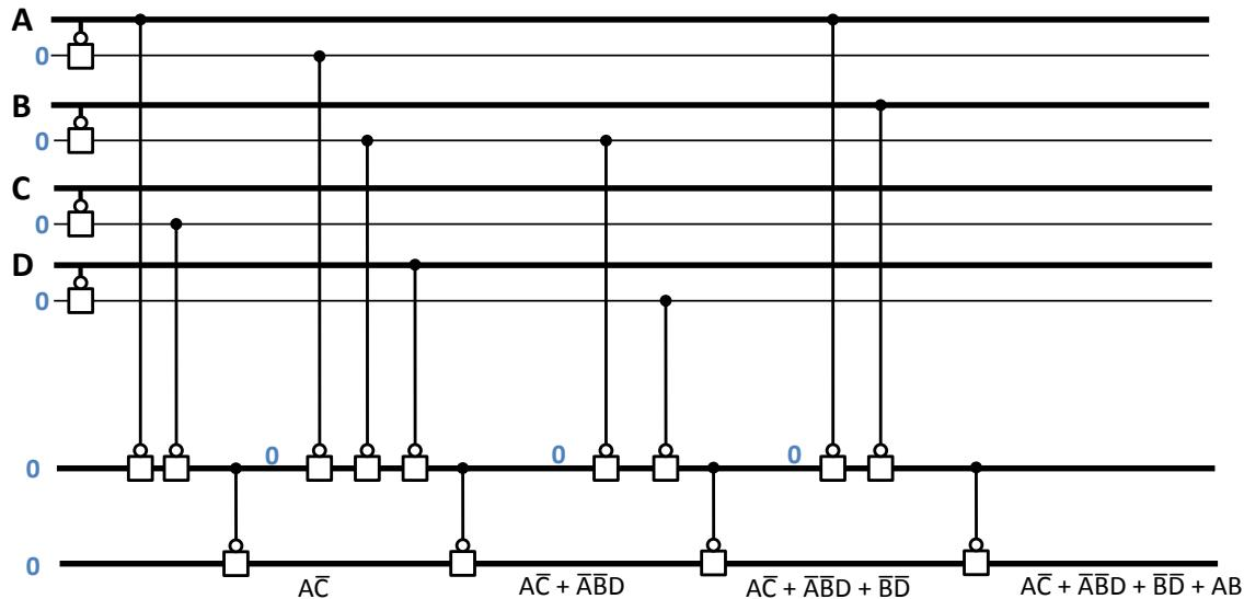
Figure 12: Realizing SOP expression  $(\bar{A}\bar{C} + \bar{A}\bar{B}\bar{D} + \bar{B}\bar{D} + AB)$  with  $N+2 = 4+2$  working memristors
