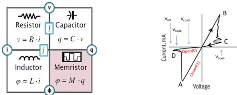
Figure 1: (a) Basic Memristor Characteristics, Source: [Strukov08],
