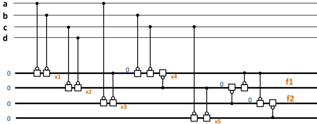
Figure 14. TANT network realized by Memristor Imply Gates
