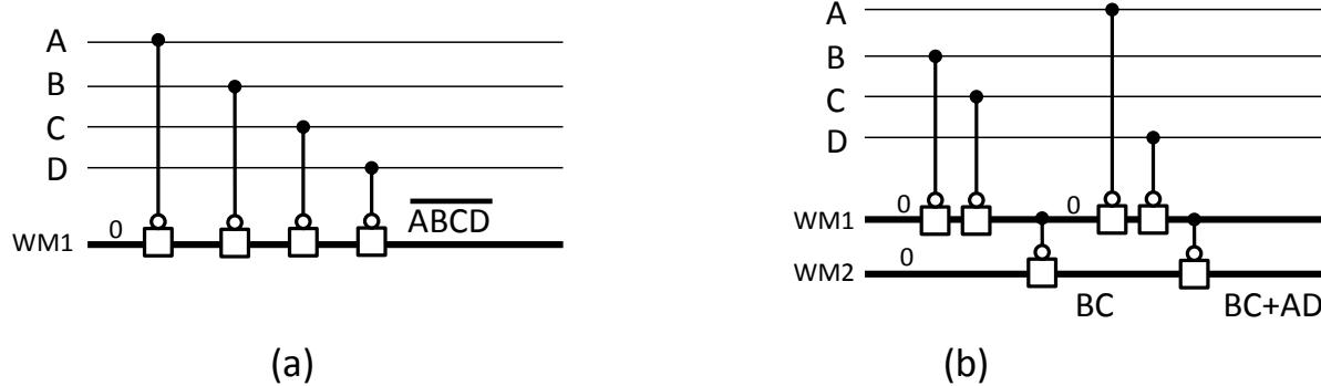
Figure 6. Imply Sequence Diagram (ISD Notation).
